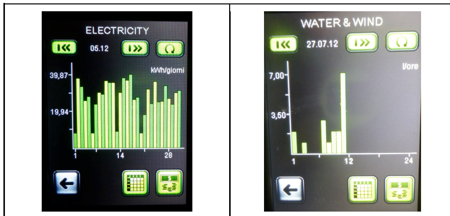
Fig. 4. Left: touch screen showing energy generated daily during May 2012. Right: water consumption on July 27, 2012 indicating waking up in the middle of night.
