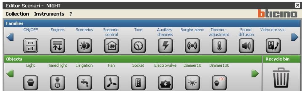
To configure a scenario, drag the object icons to the various fields below using the “drag and drop” function.
