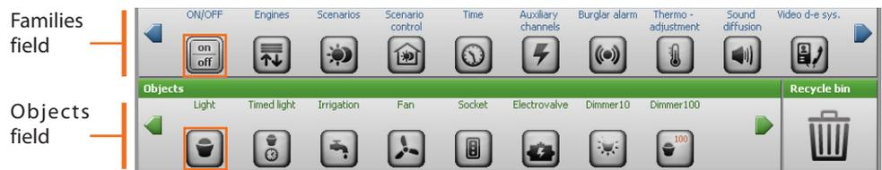
Dragging the Object (e.g.: Lamp) by means of “drag and drop”, to the relevant Field (e.g.: when it happens), when the mouse button is released, a mask is opened for the configuration of the dragged Object.
